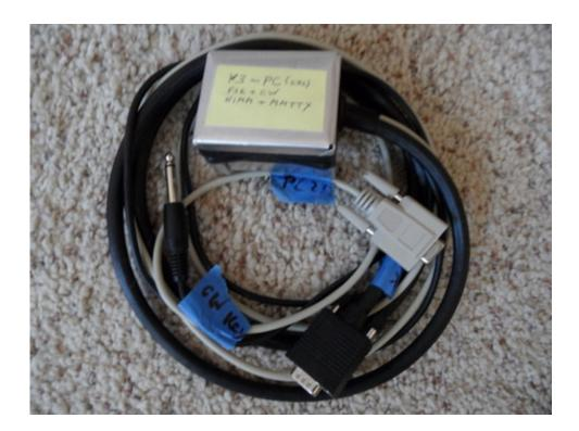
Of course, for operation the serial connector goes to the PC RS232 port, the AUX connector connects to the K3 ACC port and the phono plug goes to the K3 KEY jack.
